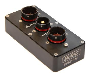
MoTeC's 16 output Marine Power Distribution Module is a fully sealed version of the PDM16 and is rated to IP68. It is designed to provide electronically switched power, in the most extreme environments, to the various electrical systems in the vehicle such as motors, lights and solenoids, and electronic devices such as ECUs and data acquisition systems.
