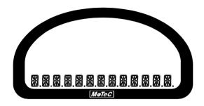
The 13 digit alpha numeric display can display up to 20 lines of information that can be scrolled up or down using the external buttons. Each of the 20 lines can display up to 3 channel values at a time.
