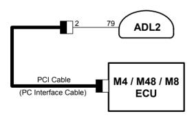
To connect a PC to the ECU disconnect the Computer Interface Cable from the ADL2 and attach it to the PC.
