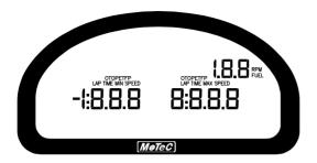
The three numeric displays (Left, Right and Top Right) can be programmed to display any value, which may be different for each of the display modes (Race Practice and Warmup).
