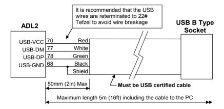
Note: When inserting the pins into the Autosport connector check that all the pins are latched correctly by pulling on each wire – it is very easy for a pin not to latch correctly which will give an intermittent connection.
